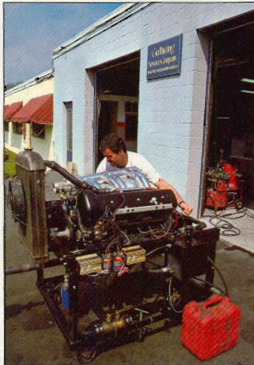
A 300 SL engine, mounted on a test stand, is tuned and run-in prior to installation in the car. A dynamometer session, and 500 to 800 miles of road testing, will precede the final O.K.
